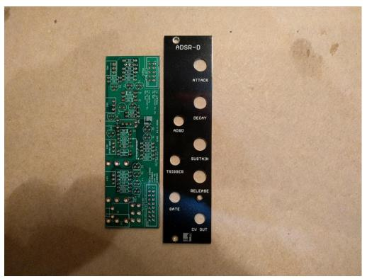
The module is designed and sized for **Eurorack** systems. You will need a 16-10 pin eurorack power ribbon connector with -12/0/+12 which is connected to a synth power supply.
